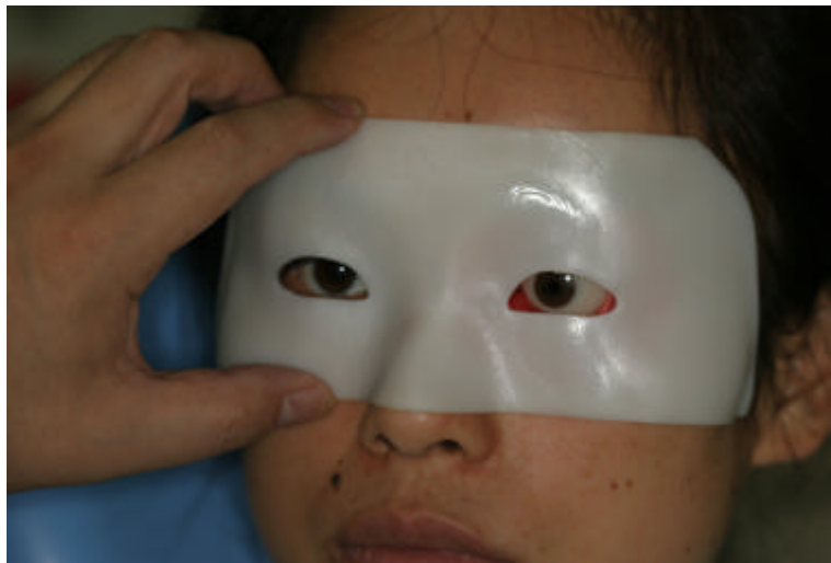
Fig. 3 The resin model manufactured by the rapid prototyping has a smooth surface and fits the patient face very well.
